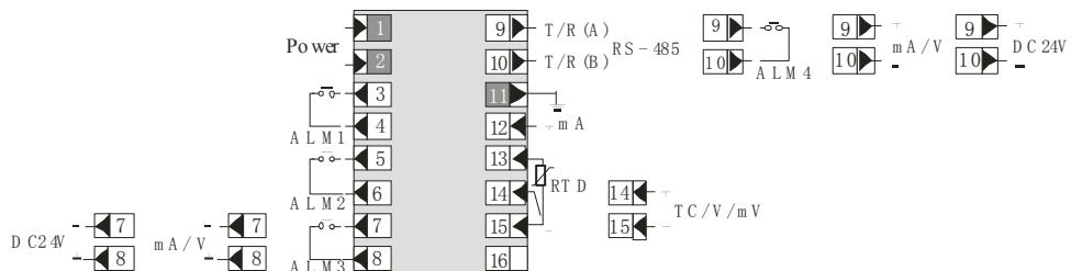
★ Note1: when have communication the transmission output locate 7、8 terminal; no communication the output locate 9、10 terminal.
