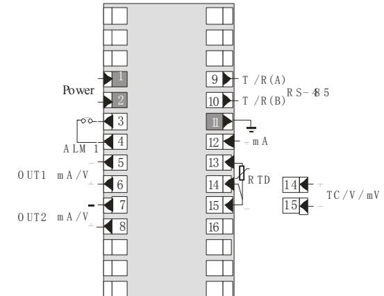
★ Note: takes the vertical wiring diagram to rotate contra-clockwise 90° immediately is 160×80 horizontal table wiring diagram.
