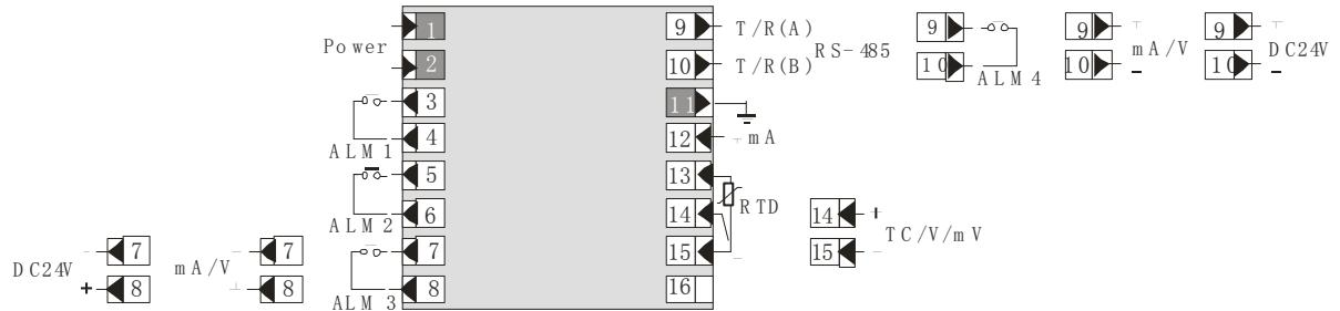
★ Note: 90 series universal type different function combination and wiring terminal arrange see table 3.
