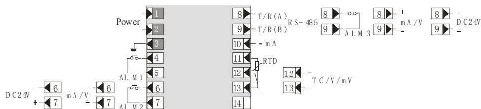
★ Note: when have communication the transmission output locate 6、7 terminal; no communication the output locate 8、9 terminal.
