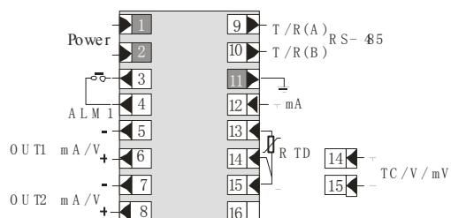
★ Note: take the vertical wiring diagram to rotate clockwise 90° immediately is 96×48 horizontal table wiring diagram.
